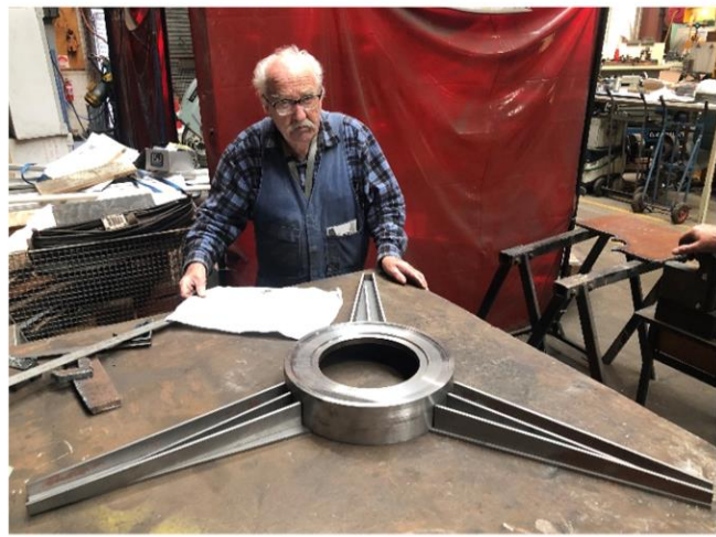
Peter finishing off the Polar Axis Movement Course Control (Slewing) small bevel gear
