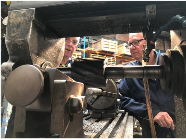
Laurie is milling the Declination axis movement course control (slewing) Handwheel Shaft as Tom watches on.
