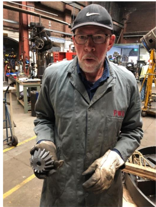
Peter finishing off the Polar Axis Movement Course Control (Slewing) small bevel gear
