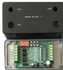
Secondary Mirror Controller (SMC) Microcontroller and Motor Drivers
