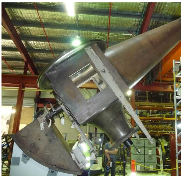
The mounting of the Great Melbourne Telescope at Moreland in 2014. Note the “cube” and the adjustable levers which could reduce the friction on the declination axle.
