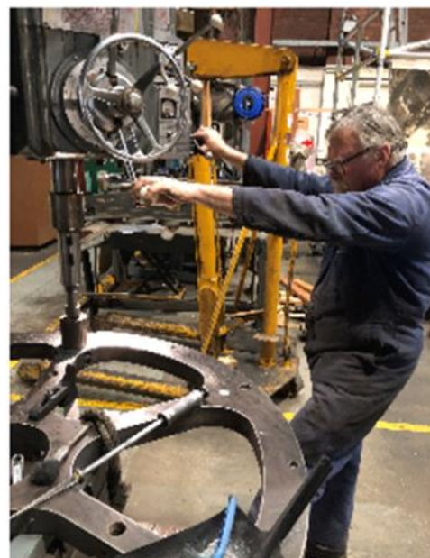
Des working on the Primary Mirror Cell Set Downs for lifting frame attachment
