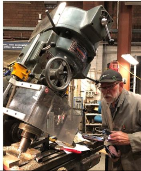
Peter machining the slide mechanism for clockwork drive.
