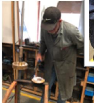
Peter heating one of the Clockwork Drive gears, to create a firm fit onto the
