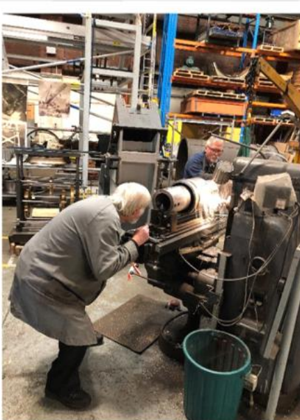
Declination Extension Tube – Eric machining slot for Encoder Cabling.
