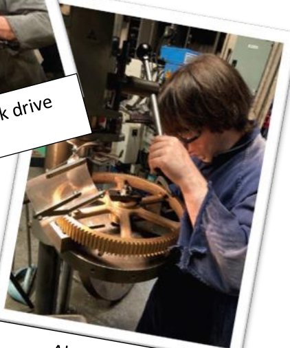
Alan D. drilling repositioned holes for the clockwork drive ratchet paws into one of the large 120 teeth gears.
