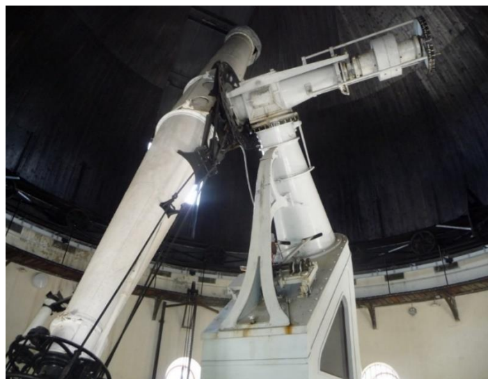
The Grubb 27-inch (69 cm) Vienna Refractor. Again, note the similarities in the mounting to the Great Melbourne Telescope.
