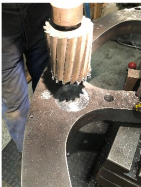
Des working on the Primary Mirror Cell Set Downs for lifting frame attachment
