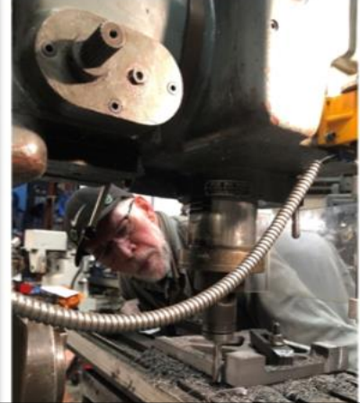
Peter milling one of the clockwork drive frames.
