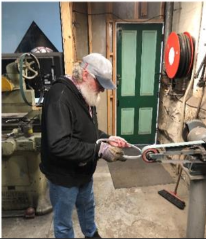
Alan W. grinding the secondary mirror baffle mounting ring.
