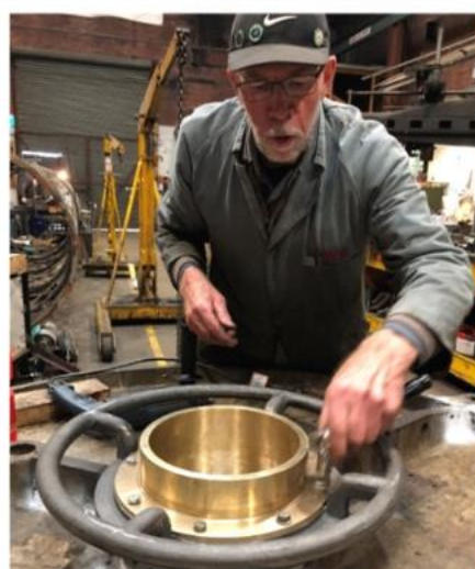
Peter finishing the focusing hand wheel assembly.
