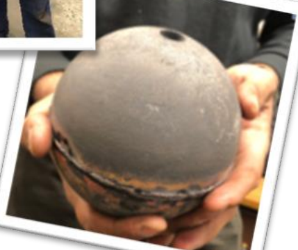
The two hemispheres welded together waiting to be filled with lead.
