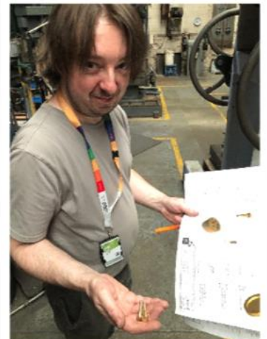
Alan D. showing the slotted cheese head screws he made for the clockwork drive upper bearing.
