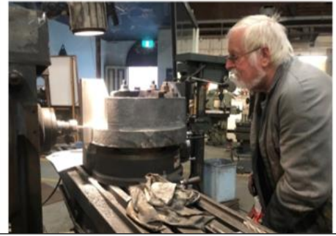
Eric continuing machining of the north bearing support
