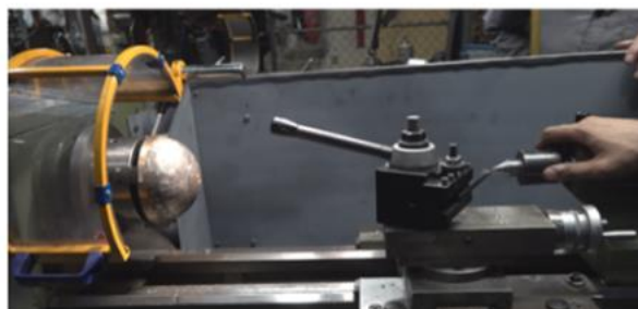
One half of the shell for the clockwork drive governor balls ready for machining.
