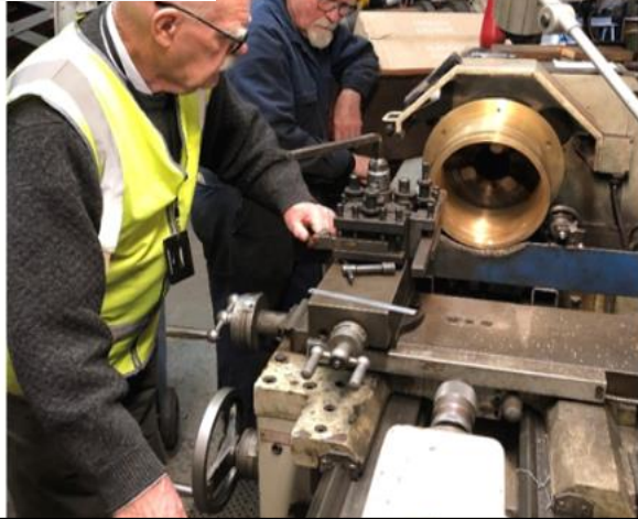
Barry and Des re-machining the mounting stub for the turret.
