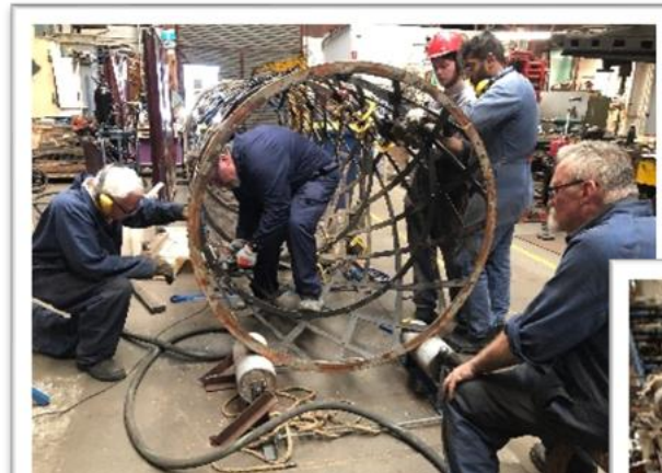
Riveting of the secondary ring to the lattice tube.
