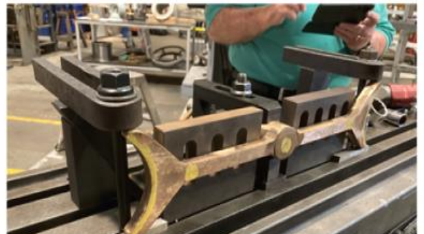
The rest stop for the governor balls in the clockwork drive is set up for machining.
