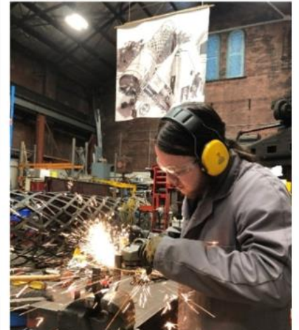
Oscar grinding the Sidereal / Lunar clutch lever plate.
