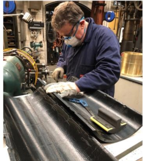
Stewart preparing the mould for the carbon-fibre baffle.
