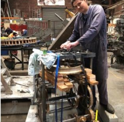
Horatio tapping holes in the clockwork drive top plate.
