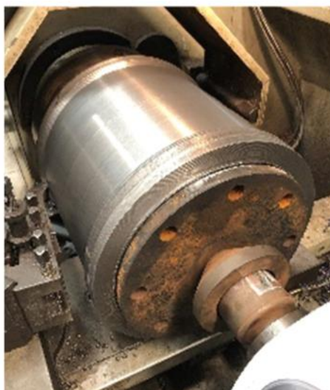
The Clockwork Drive drum beginning to be machined.
