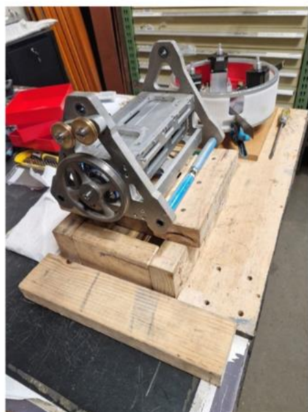
Secondary Mirror Cell being assembled.
