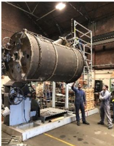
The Boiler Plate Tube balancing for dynamic testing.
