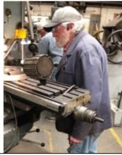
Alan W. drilling the secondary mirror cell balancing weight.
