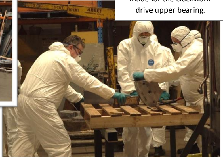
The "lead team" shaping the counterweights.
