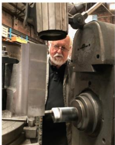
Eric machining fillets on the north bearing support.
