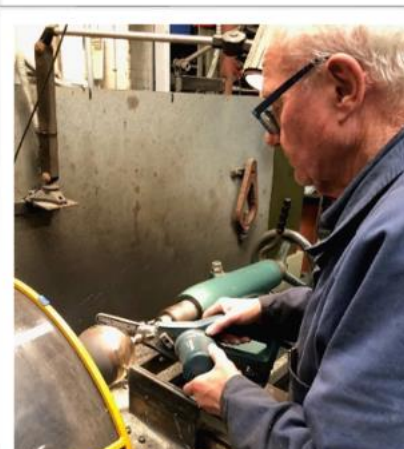
Tom showing off a secret method of machining the clockwork drive governor balls.
