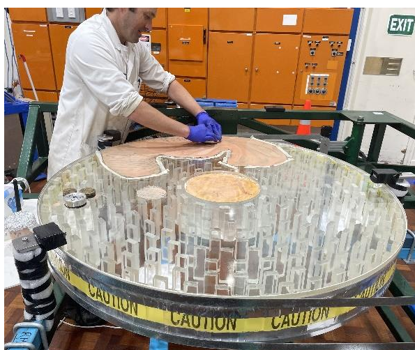
Hand polishing of the GMT primary mirror to locally correct astigmatism, by KiwiStar, NZ.
