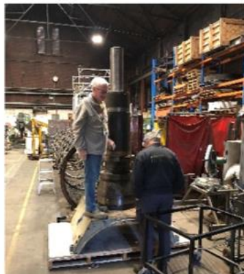
Des & Laurie disassembling the declination axis.
