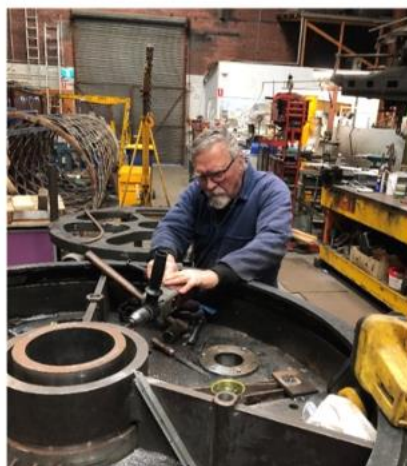
Des installing the access for the optical tube counterweight cabling.
