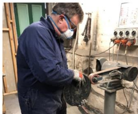
Stewart finishing off the support disks for the secondary baffle mould.
