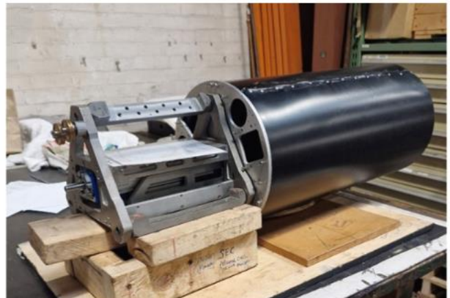
Test baffle connected to secondary mirror cell.
