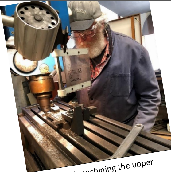
Barry re-machining optical flat bearing for turret
