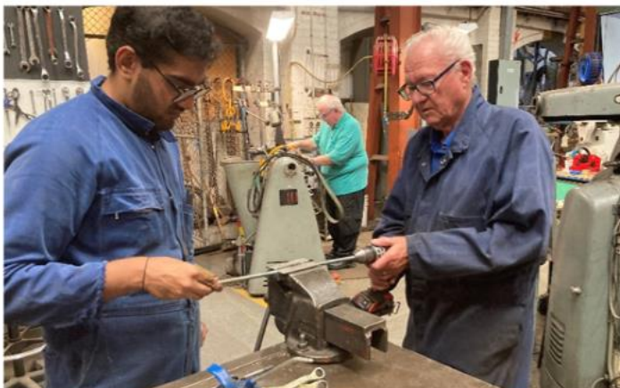
Tom and Ali preparing the mandrel for machining the clockwork drive governor balls.
