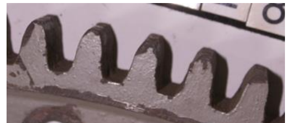
Original Grubb cycloidal tooth profile Ring Gear
